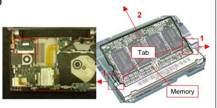
Outspread the tabs (arrow 1) and pull out the Memory obliquely upward (arrow 2).
