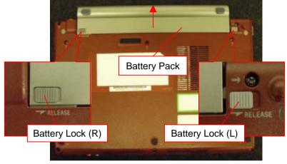
Remove the Battery Pack while moving the Battery Lock (L) and the Battery Lock (R) to the **RELEASE** side.
