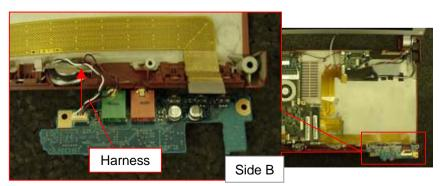
Disconnect the Harness and remove the CNX Board.
