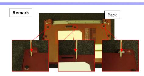
When the Keyboard can not be removed, insert the bamboo skewer from the back into the screw holes (three places) and release the keyboard.
