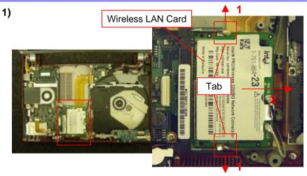
Outspread the tabs (arrow 1), and pull out the Wireless LAN Card obliquely upward (in the direction of the arrow 2).
