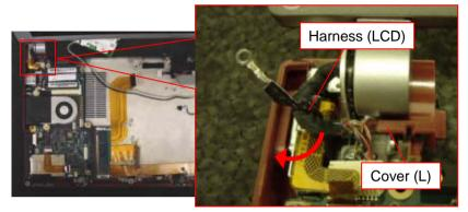
Pull out the Harness (LCD) from under the Cover (L).
