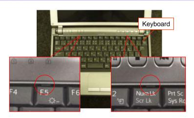
Disengage the detent (two places) and release the Keyboard. \*Push the detent with the bamboo spatula and disengage it.
