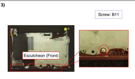
Remove the one screw and the Escutcheon (Front).
