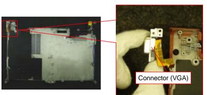
Remove the Connector (VGA).
