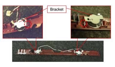
Remove the Bracket (two places) while disengaging the detent (each one place).
