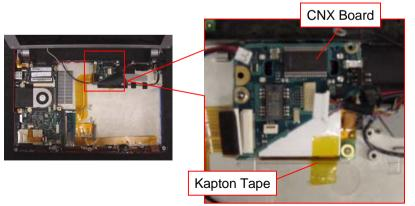
Peel off the Kapton Tape and remove the CNX Board. \*There is the Modem Card on the rear.
