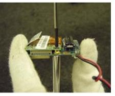
Remove the screw while securing the Nut of the side A with the 4 mm socket wrench.
