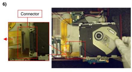
Disconnect the connector and remove the Optical Disc Drive.
