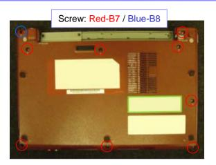
Remove the nine screws from the Bottom.
