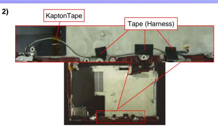
Peel off the Kapton Tape (one place) and Tape(Harness) (three places).
