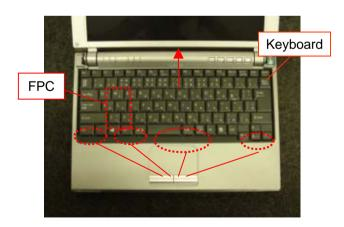
Slide the Keyboard in the direction of the arrow, disengage the detent (four places) and turn down the front side.
