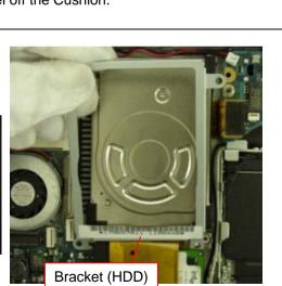
Remove the Bracket (HDD).
