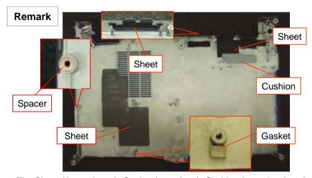
The Sheet (three places), Gasket (one place), Cushion (one place) and Spacer (one place) are attached to the Housing (Bottom).
