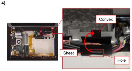
Remove the convex portion of the Sheet from the hole.
