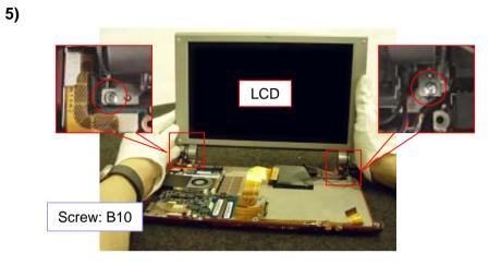
Remove the two screws and the LCD.
