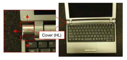
Remove the Cover (HL) in the direction of the arrow while outspreading its both sides and disengage the detent (two places).
