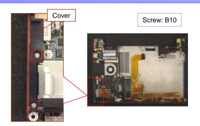
Remove the two screws and the Cover.
