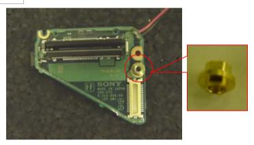
The Stand is installed under the Modem Card.
