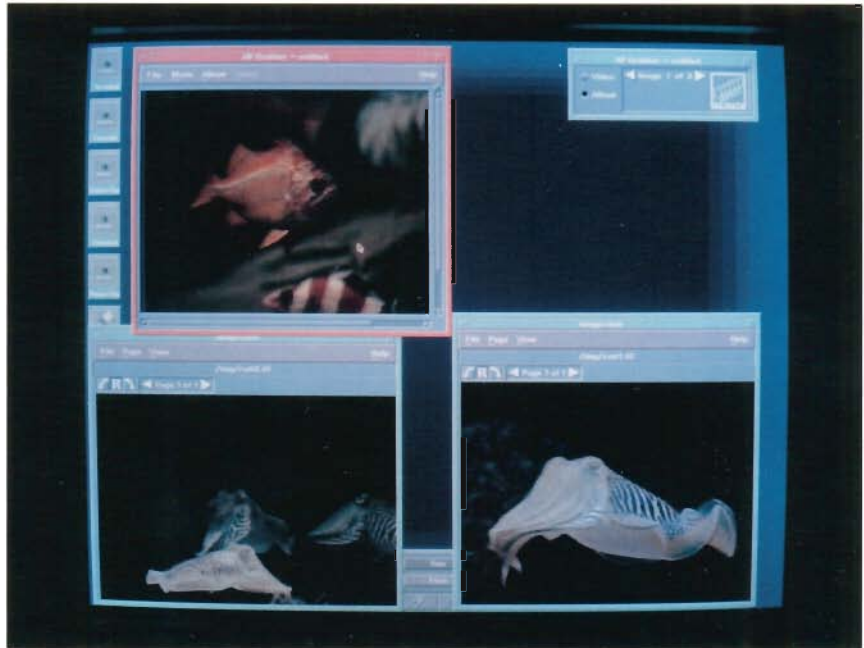
Image Analysis: an HP 9000 Series 720 workstation screen. The top left window shows an image of fish in an aquarium captured from videotape. The bottom two windows show TIFF images of previously captured frames. Users can take video tape of an event in the field, and capture the ideal frames for subsequent image analysis.
