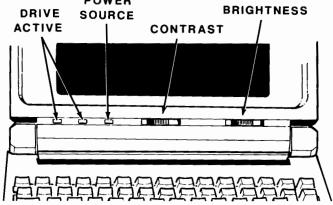
Figure 1-3. Brightness and Contrast Controls
