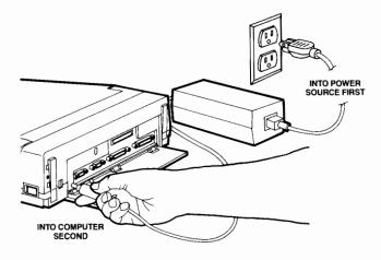
Figure 1–1. Power Adapter Connection
