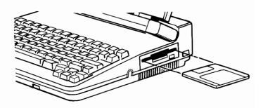
Figure 1-4. Inserting the SETUP Program Disc
