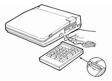
Figure 2-4. Connecting the Numeric Keypad
