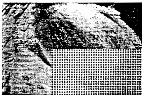
4-by-4-pixel halftone cells, spiral dither
