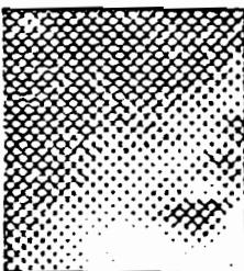
Left: Enlarged view (500 percent) of Lino-tronic 100 (1270 dpi) output at 150 lpi and 256 levels of gray. Note that the higher-resolution device produces a much finer halftone pattern without loss of gray information.
