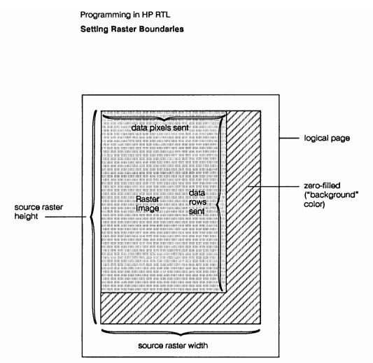
Zero Filling Using Source Width and Height
