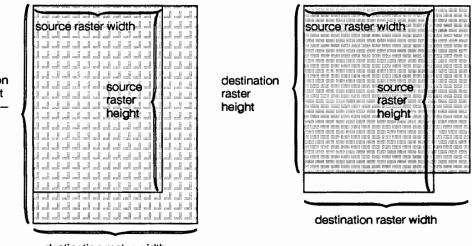
destination height not specified – causes isotropic scaling
