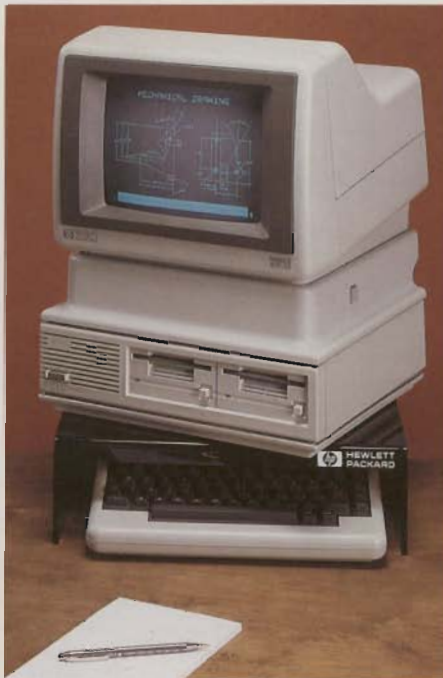
Use these convenience accessories to: (1) tilt display up/down and (2) swivel equipment right/left for easiest use, and (3) park keyboard out of the way when not in use.
