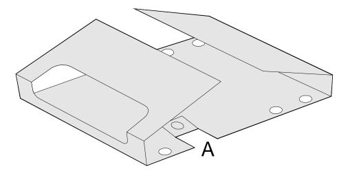
7. Holding the new hard drive by its edges, with the connectors on the left side, lay it in place. Grasp the right Mylar flap and pull to the left to engage the connection between the hard drive and the computer. Do not push down on the hard drive. If the hard drive's connectors do not
