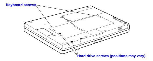
4. Remove the keyboard by inserting your fingertips between the top row of keys (the F keys) and the case and then lifting. Then fold the keyboard gently forward so that it lies upside down on the table. Do not pull up on the keyboard. Keep the ribbon cables tucked in the case, otherwise you will need to tuck them back in with a paper clip.
