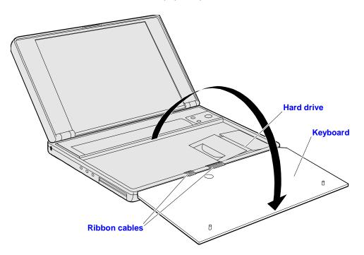
5. Handle the hard drive only by its edges to avoid damage from electrostatic discharge.
