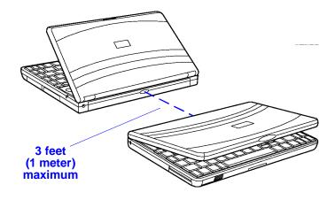
2. Start the IR Monitor: click Start, then Infrared. This activates the connection between two IrDA-compatible infrared ports.
