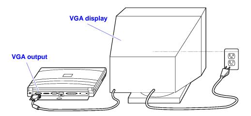
The OmniBook automatically recognizes and activates the external display. The built-in display normally turns off to conserve power and backlight life. If you keep it on, you may notice a slight dimming while the external display is connected.
