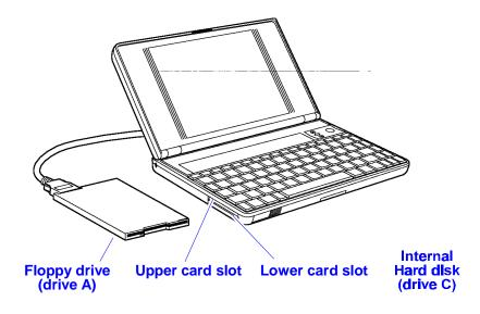
You can use the upper and lower card slots with plug-in PC cards much as you now use floppy disks. You can plug in a PC data-storage card and write data to it or read from it just as if it were a floppy disk.
