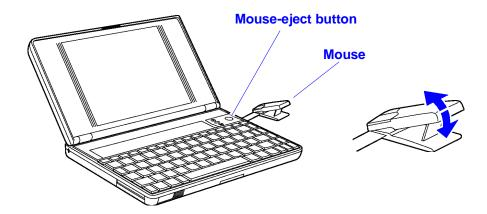
The mouse is extremely sturdy. Its flexibility allows it to withstand bending and accidental bumps without breaking.
