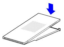
4. Slide the tray fully into the slot and secure its latches.
