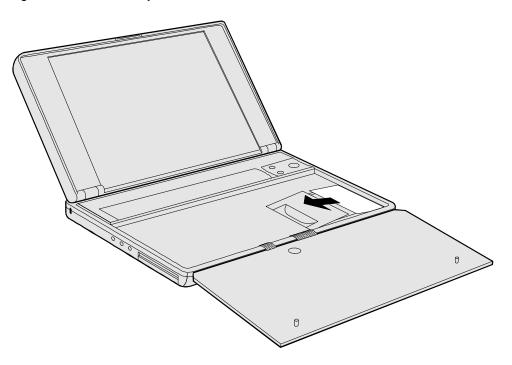
8. If the ribbon cables are no longer tucked into the frame, then push them back into the recessed openings with a paper clip, as shown below. Reinsert the keyboard by engaging the four front tabs on the keyboard into the four slots in the computer frame, pressing down on the keyboard as you insert the tabs. Make sure the ribbon cables slide into the recessed openings and do not extend under the keyboard.
