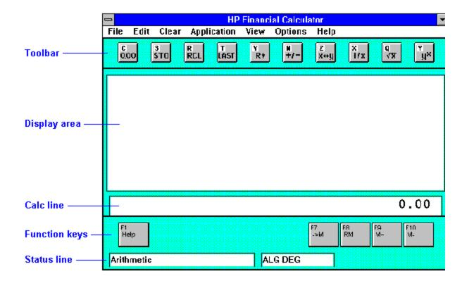
HP Calculator "takes over" part of your OmniBook's keyboard and reassigns functions to it. You can see these functions and the applicable keys on the display of calculator buttons—for example, pressing the Q key takes the square root of the number in the Calc line.
