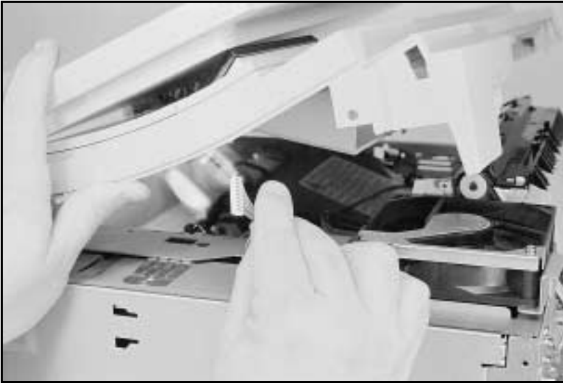
Figure 6-4 Control Panel Cable
