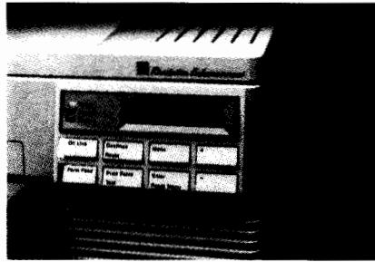
LCD on printer front control panel shows that the optional Adobe PostScript cartridge is installed.
