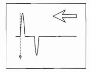
Figure C-6. Lining up the outgoing pulse
