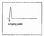
Figure C-1. No cable attached
