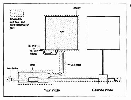
Figure 12-4. Self Test coverage on a ThickLAN
