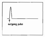
Figure C-10. LAN cable unconnected
