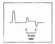
Figure C-8. 75 Ohm Cable Between 50 Ohm Cable, Without MAUs/ThinMAUs
