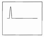
Figure C-5. MAUs, reversed polarity
