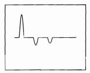
A test with the polarity reversed also shows what we expected: the negative pulses disappear, indicating that they were caused by MAUs. Everything looks O.K., so we make a strip chart record of this display, too. We store both strip charts in the file with the other records for this LAN cable; that gives us a base record for comparison if we have problems with this LAN cable at some later time.
