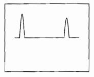
This time the LAN cable passes the re-test. Now we use the TDR to make a record of the functional cable. A normal polarity TDR test shows just what we expect to see: negative pulses at the locations of the two MAUs. We use the strip chart recorder of our TDR to make a permanent record of the state of the LAN cable.
