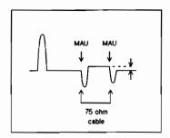
Figure C-9. 75 Ohm Cable With MAUs/ThinMAUs Installed on Each End
