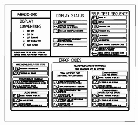
Figure 12-3. Self-Test and Error Code Label
