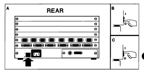
Figure 12-1. DTC Power Switch Operation
