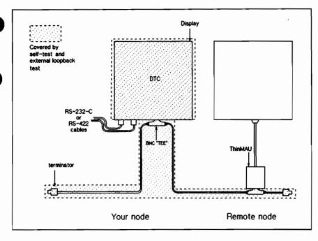
Figure 12-5. Self Test coverage on a ThinLAN
