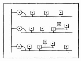
Figure B-1. Two HP 92223A's Max Between Nodes
