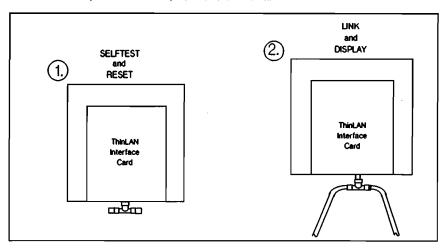
Figure 11-4. Internal - External error testing
