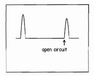
Figure C-2. Open circuit
