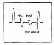
Figure C-12. Open circuit
