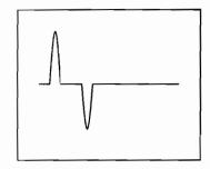
We reverse the polarity and test the cable again. Suspicions confirmed: it is a short circuit at the location of the first MAU. (If the negative pulse had been caused by the MAU, the pulse would have disappeared when we reversed the polarity.) We do a continuity test on the first MAU and find a short circuit, so we replace the MAU. Subsequently, the cable is retested in accordance with the procedures.
