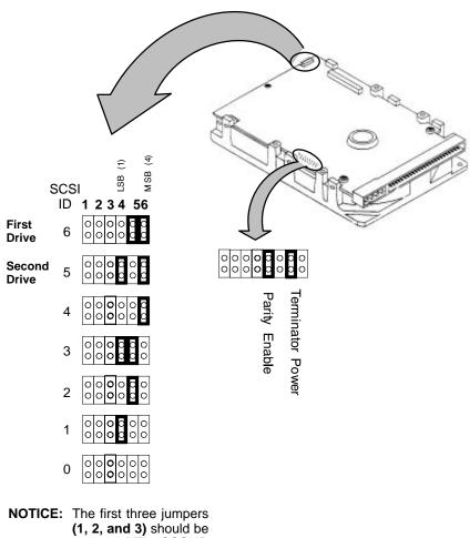
NOTICE: The first three jumpers (1, 2, and 3) should be removed. The SCSI ID jumpers are jumpers 4, 5, and 6.
