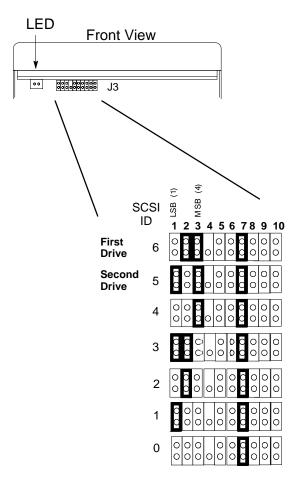
NOTICE: The first three jumpers (1, 2, and 3) are the SCSI ID jumpers. The only other jumper that should be *in place* is 7. These are the only jumpers that should be installed.
