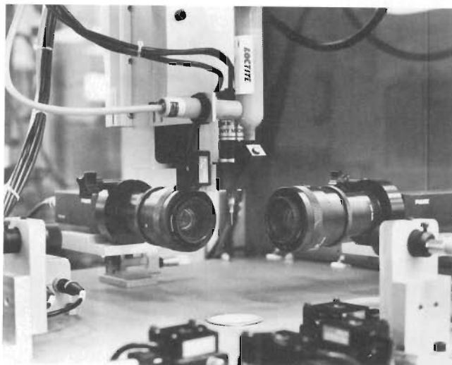
Fig. 2. The adhesive and encapsulant dispensing stations are equipped with two orthogonally positioned cameras using back-lighting to determine the position of the dispensing needle tip accurately.
