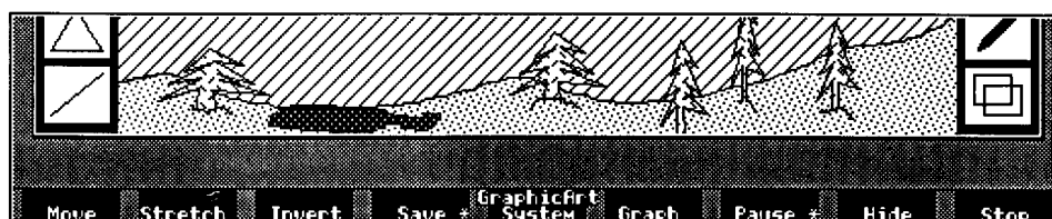
Fig. 2. View of system menu along lower portion of the display. An asterisk is displayed for one of the two states in label blocks for toggled modes. (Save and Pause in this example).
