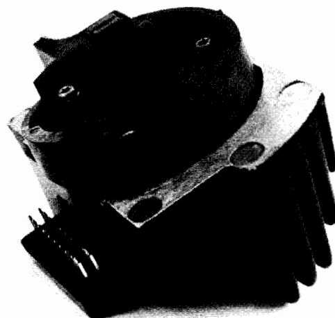
Fig. 2. (a) Configuration of the printwires on the HP 293X printhead as viewed looking through the printhead to the surface of the paper. (b) Photograph of printhead.
