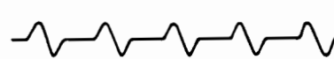
Fig. 5. Format of the servo surface, a surface in the center of the multidisc pack dedicated to track position information.
