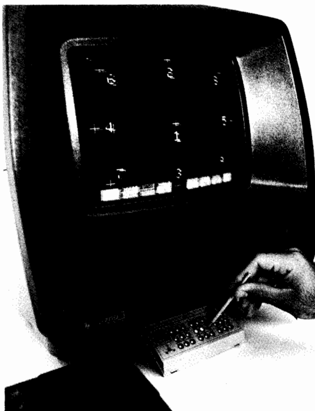
Fig. 2. For convergence adjustment, color-coded potentiometers behind a swing-down panel are adjusted while watching a target pattern on the screen.
