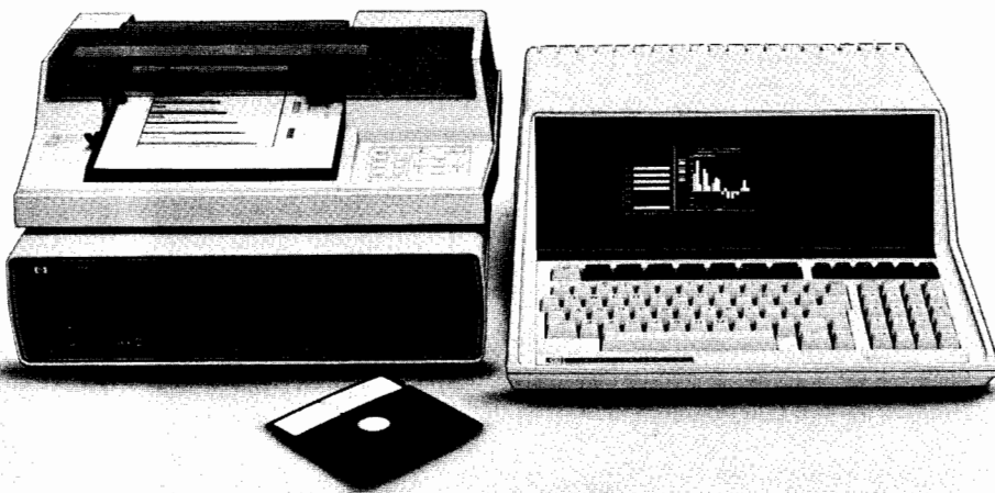
Fig. 3. The HP-87XM Computer is the premier member of the Series 80 family. It features a built-in CRT display and an HP-IB interface for communication with disc drives, printers, and plotters. Its large (128K bytes) internal user memory can be expanded up to 640K bytes by adding RAM modules to its four expansion ports.
