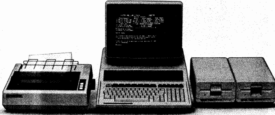
Fig. 2. The HP-86 Computer is the nucleus of a modular computer system. It can drive up to two HP 9130A flexible disc drives and a Centronics-compatible printer directly with its built-in interfaces. Video output is displayed on an external monitor. Both 9-in (82912A) and 12-in (82913A) monitors are available from HP.
