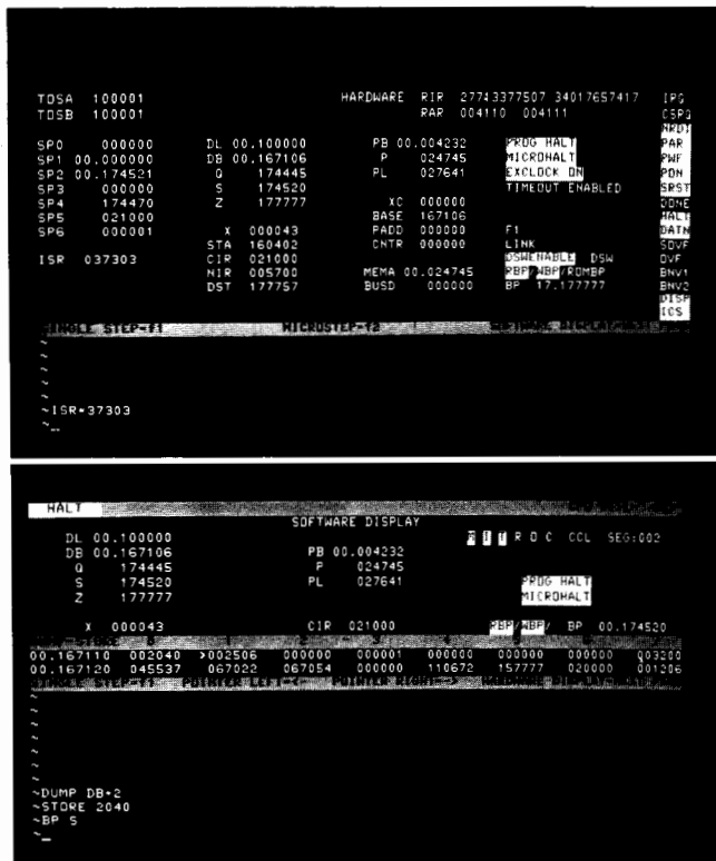
Fig. 3. Maintenance displays on local and remote consoles show CPU registers, flags, and memory information.
