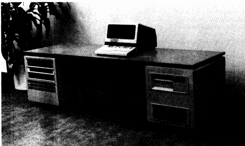
Fig. 1. HP 3000 Series 33 Computer System. Base model includes a 20M-byte cartridge disc drive, 256K bytes of fault-control memory, seven ports for 2400-baud asynchronous terminals, two general I/O channels, and a one-megabyte double-sided flexible disc drive. The Series 33 runs the same Multiprogramming Executive operating system (MPE III) as the more powerful HP 3000 Series II and Series III systems, and will execute Series II and Series III application programs without changes or recompilations.
