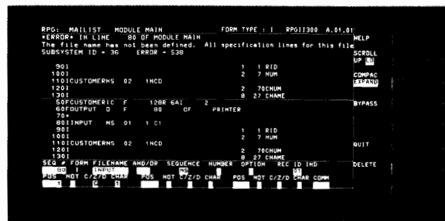
Fig. 5. When the TEST softkey is pressed, compilation begins. If an error is discovered, it is displayed on a split screen. The user can correct the error, BYPASS it temporarily, or QUIT the error processing mode.
