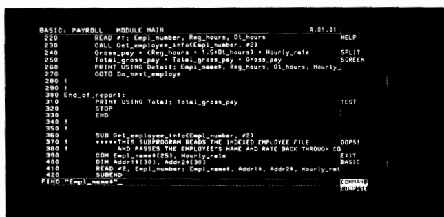
Fig. 5. The IDS screen while the BASIC language subsystem is in command mode.
