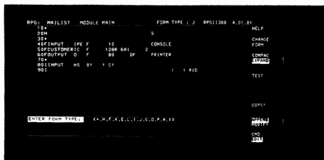
Fig. 3. To switch templates the user presses the CHANGE FORM softkey, and is offered a menu of form types.
