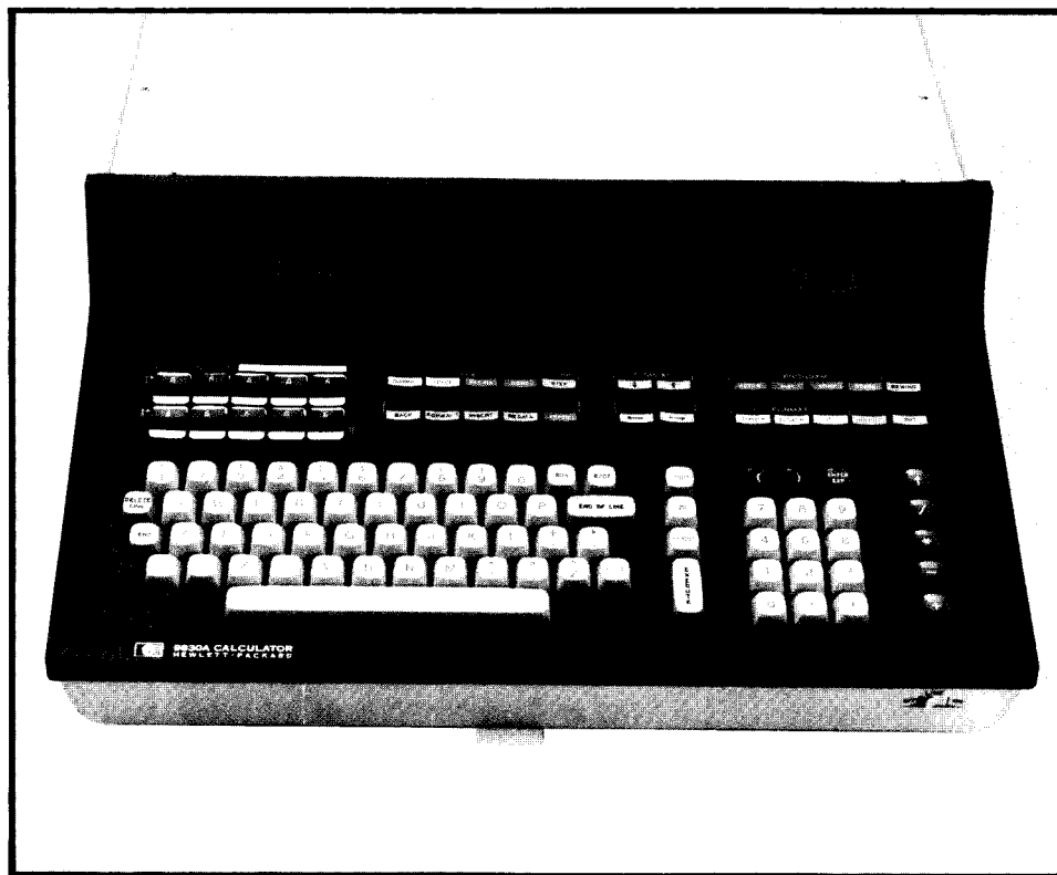
Fig. 1. Model 30 of the 9800 Series has an alphanumeric keyboard like a teleprinter. Its language is BASIC. It can be used as a desktop computer or a remote computer terminal, yet it maintains the convenience and user interaction of a programmable calculator.
