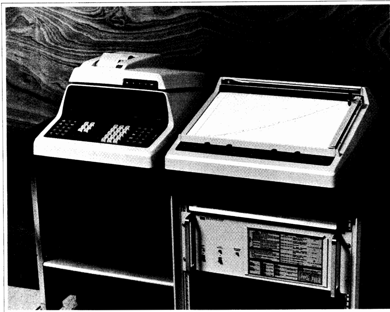
Fig. 1. This Hewlett-Packard Model 9101A Extended Memory attaches directly to the Model 9100A/B Calculators. It adds 248 registers of memory greatly increasing the computing power of the calculators.
