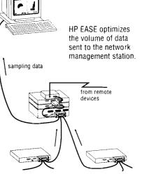
HP EASE distributes embedded instrumentation throughout the network.
