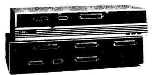
The HP 28688B EtherTwist Hub Plus and HP 28699A EtherTwist Hub Plus/48 are 10Base-T multiport repeaters that include 12 or 48 twisted-pair ports, 1 thin coaxial (BNC) port and 1 AUI port. The Hub Pluses repeat and retime signals, handle collision management, and monitor individual link status. In addition, the hubs automatically segment individual ports disturbing the network and reconnect them when the problems are cleared.
