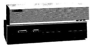
Using the same form factor as the HP EtherTwist Hub Plus/48, the HP 28692A ThinLAN Hub Plus provides added functionality to HP's "rack-and-stack" family of network components. The HP ThinLAN Hub Plus is a manageable, multiport, thin-coaxial repeater for use in Ethernet and IEEE 802.3 local area networks. With nine thin coaxial (BNC) ports and one AUI port, this SNMP-based hub provides a scalable, manageable, and flexible solution for 10-Mbit/s LANs using thin coaxial cable.
