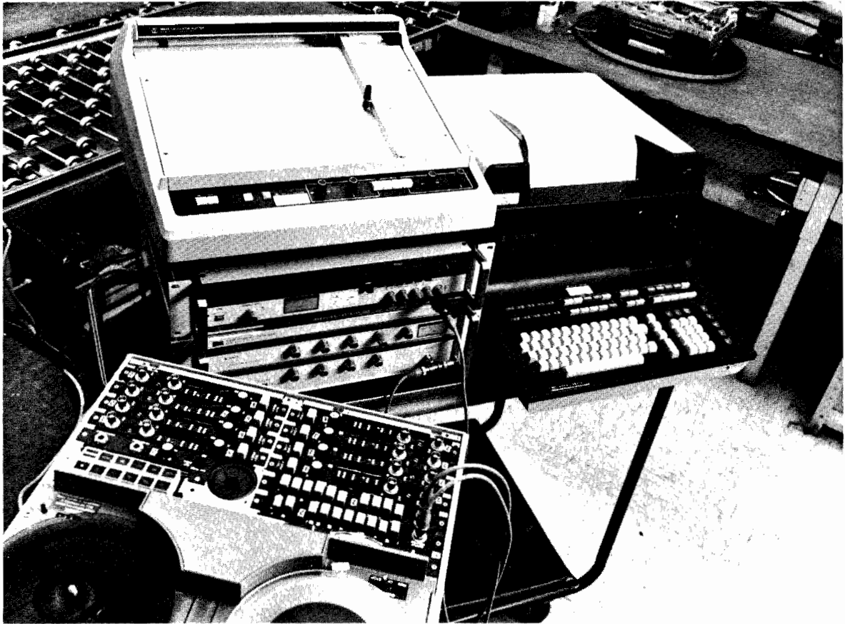
FIGURE 5. SEMI-AUTOMATIC SYSTEM FOR PRODUCTION AND ENVIRONMENTAL TESTING OF TAPE RECORDERS. THIS PORTABLE AND COMPACT SYSTEM INCLUDES A CALCULATOR AND PRINTER; A FREQUENCY SOURCE; A DIGITAL MULTIMETER; AND A PLOTTER. UNIT UNDER TEST (LEFT FOREGROUND) IS AN INSTRUMENTATION TAPE RECORDER.
