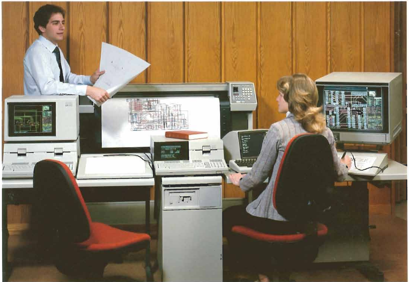
EGS/200 runs on HP's Shared Resource Management (SRM) system; shown is a typical workstation configuration (left) and a typical large-display configuration (right).
