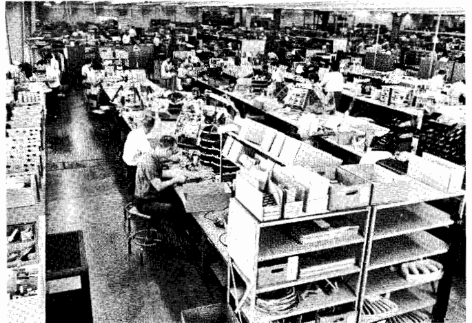
RF wiring and assembly line. While adequate for Dymec's volume in the past, modernized layout will streamline parts and work flow, cutting down wasted movement. Production volume for given floor space will be increased.
