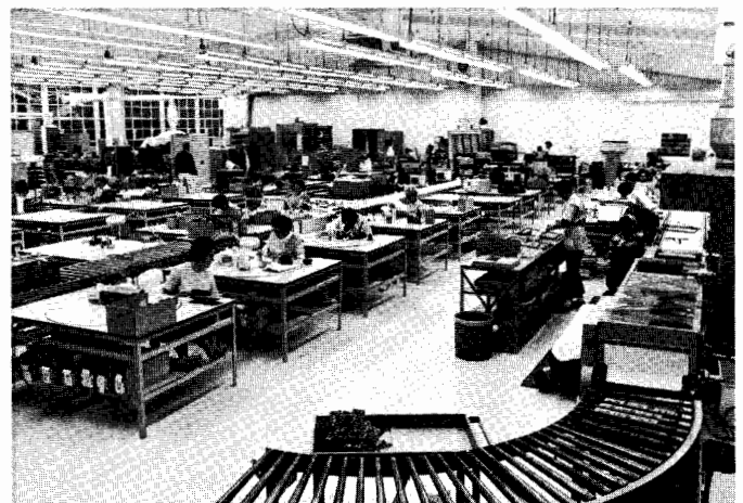
Photo shows new semi-automatic, flow-soldering machine at right. Soldered boards pass through fully-automatic washing machine and are delivered by roller conveyer (section is missing in immediate foreground) to touch-up and secondary assembly line, finishing up in pre-fab test area at back of room. New work benches allow parts to be stored off floor, are at normal desk height.
