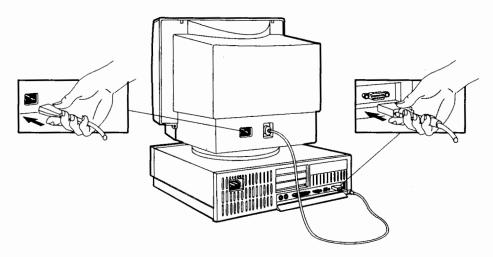
This display has been designed to operate on all power systems, including "IT" power systems. It is disconnected from the power by removing the power cord from the power outlet. This means the display must be located close to a power outlet that is easily accessible.
