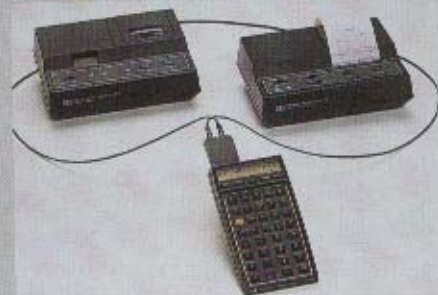
(L): HP-IL concept; (R): HP-41 computer/controller on the HP-IL with 82161A digital cassette drive and 82162A thermal plotter/printer.
