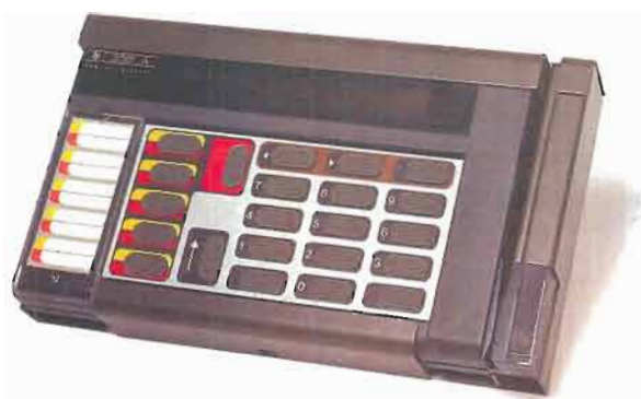
3081A with numeric keyboard, bar code slot reader, and mounting bracket.
