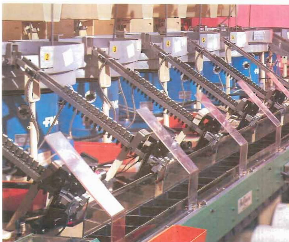
HP's plotter pens are packaged in a specially coated foil bag, then heat sealed along the edges. This creates a moisture barrier to prevent pens from drying out, which ensures fresh pens and a long shelf life.
