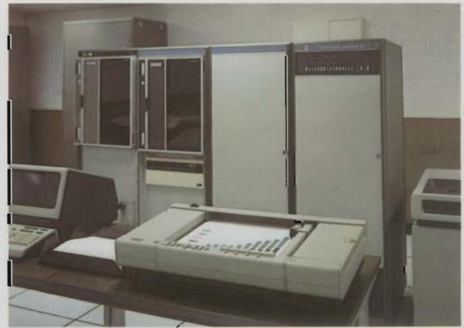
Figure 5. An HP 7221S plotter with paper advance capability is used to output data from a large computer system - a data display application.
