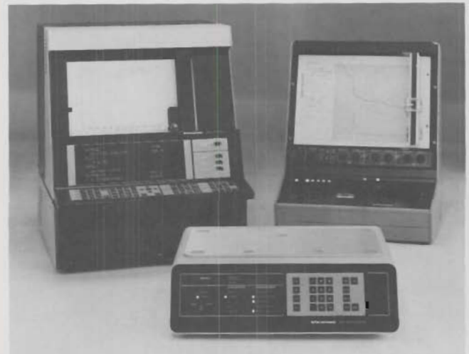
Figure 6. ▲ An HP plotter and an HP X-Y recorder are integrated into this Dupont thermal analysis system.
