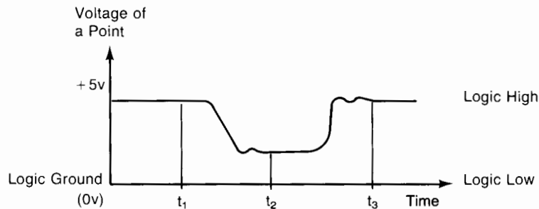
Figure 2-9. Voltage and Positive-True Logic
