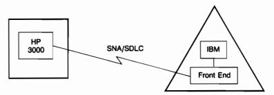
The same types of SNA emulation that are done through the SNA gateway are also available as standalone products: SNA IMF for interactive access, SNA NRJE for batch job submission, and LU 6.2 Base (together with HP Office-Connect to DISOSS) for electronic mail exchange and DISOSS library access. An SNA Link is required on each system and all three of the above products can be supported on the same system over the same link.
