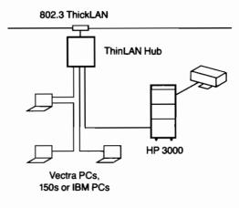
HP ThinLAN runs at 10 Mbps and offers an alternative to HP StarLAN in technical environments that require office automation solutions in addition to technical applications.
