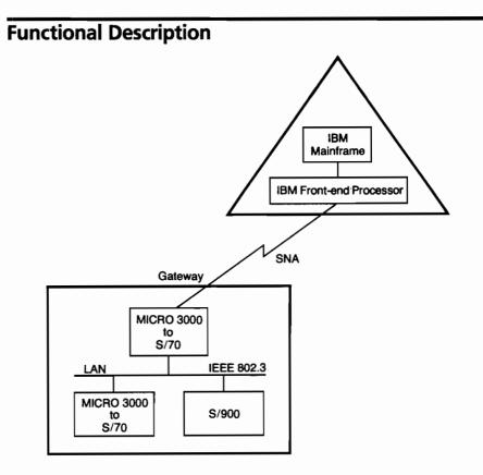
The picture shows two HP 3000 systems accessing an SNA Gateway to IBM. The gateway provides SNA batch job submission, SNA interactive access to 3270 applications and SNA LU 6.2 access to DISOSS for electronic mail exchange to/from HPDesk users.
