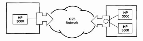
By running the NS 3000/V Network Services, terminal users and software processes can open multiple sessions to remote locations. They can logon to remote systems, transfer data and access remote files, data bases and peripherals. An X.25 line concentrator can be used to allow several systems to share one single access line to an X.25 network. HP 3000 computers can communicate over public and private X.25 networks.
