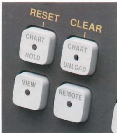
Just four front-panel buttons control normal plotter operation.
