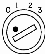
Drive Select Switch (Shown Set to 0)
