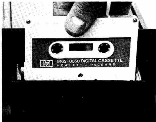
Figure 2-3. Inserting a Tape Cassette
