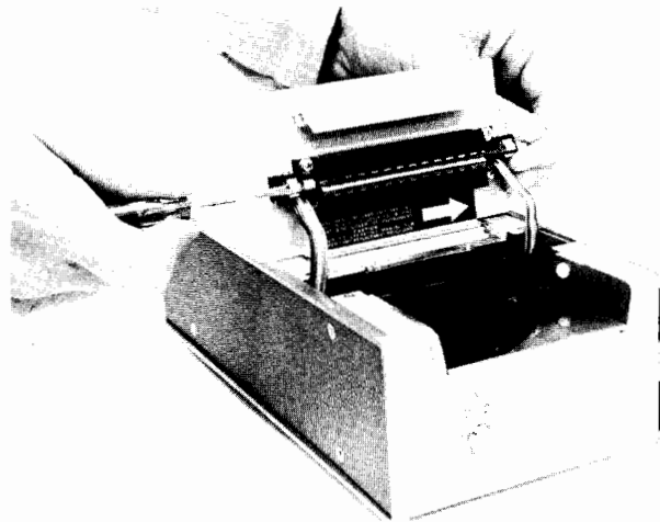
Figure II-9. Removing the Old Lamp.
