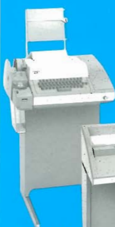
Option R00 Teleprinter* (10 char/sec 72 char/line)
