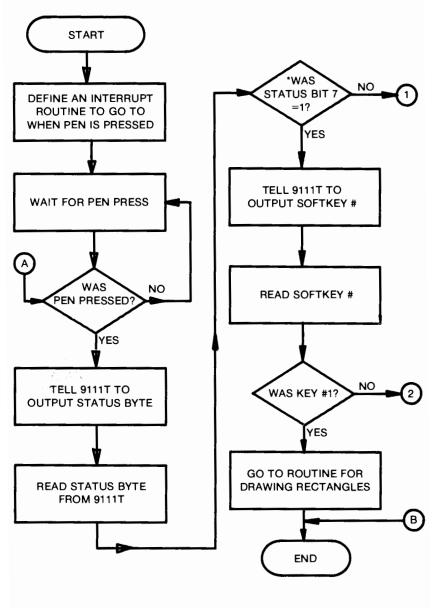
Figure 3-8. Interrupt Routine Flowchart
