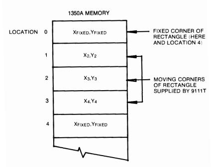
Figure 3-5. 1350A Memory Configuration When Using EE4 Command.
