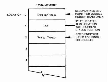
Figure 3-2. 1350A Memory Configuration When Using EE1 Command.
