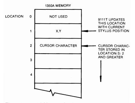
Figure 3-1. 1350A Memory Configuration When Using EE0 Command.
