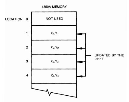
Figure 3-6. 1350A Memory Configuration When Using EE5 Command.
