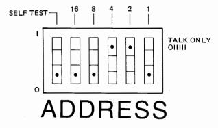
The following table lists the ADDRESS switch positions for each address code value.
