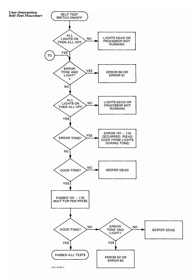
\*ERROR light comes on after tone sequence when using SELF TEST switch and during tone sequence when using TD.
