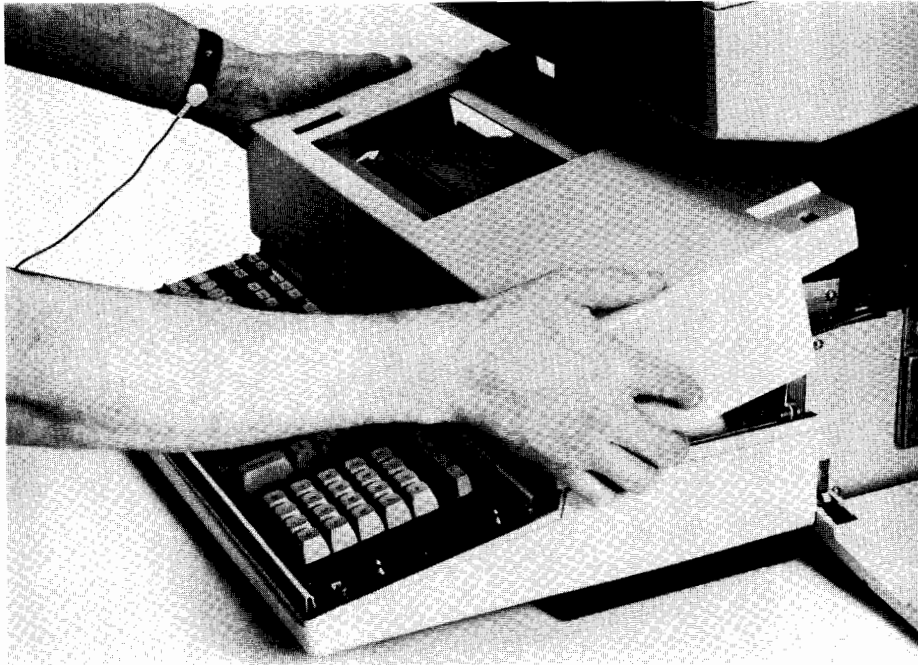
Figure 4-6. Removing Front Cover
