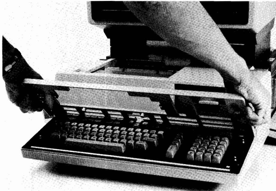
Figure 4-4. Removing Keyboard Bezel
