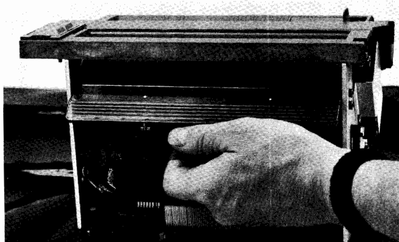
Figure 4-37. Removing Transparent Cover
