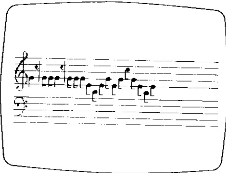
This display shows just how versatile and sophisticated the HP-85 graphics system can be. The staves, clef marks, notes and rest marks were all drawn with the user-definable graphics operations.
