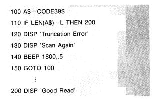
Scans and decodes bar-code label. Compares its length to L, the known field length. Displays error message if lengths aren't equal.
