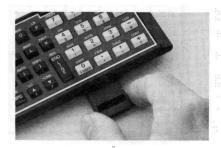
To remove the module, use your fingernail to grasp the lip on the bottom of the front edge of the module and pull it straight out of the port. Install a blank module in the port to protect the contacts inside.
