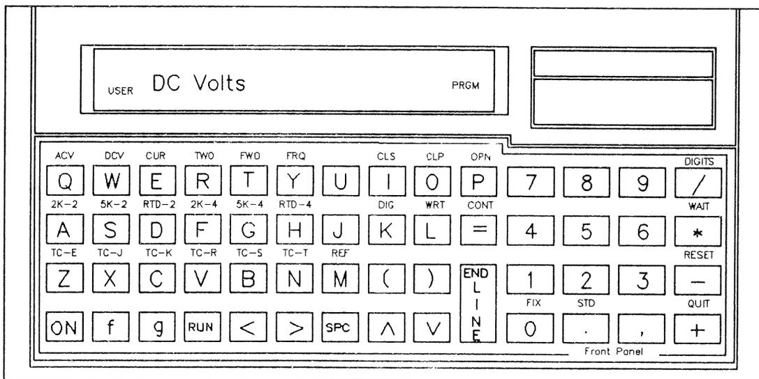
The identity of each command key is shown *above* the key on the overlay. For example, to select DC Volts, press [**DCV**] (the **W** key). To select AC Volts, press [**ACV**] (the **Q** key). For convenience, each command key will be identified in this section by its name on the overlay.
