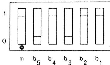
The HP-IL/HP-IB interface switches configured for *mailbox* mode at HP-IB address 11.
