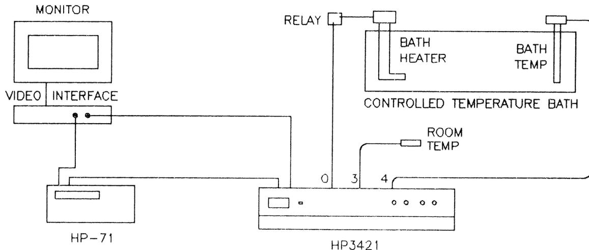
Figure 7-2. Temperature Monitoring System With Actuator Control
