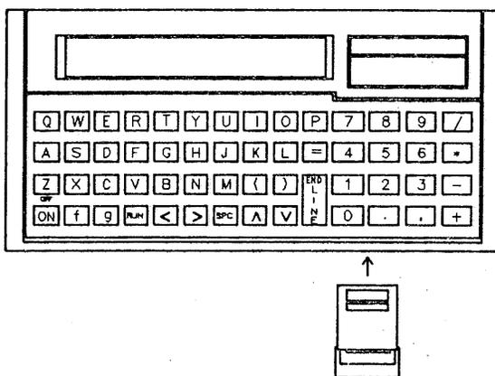
To insert the module, hold the HP-71 with the keyboard facing up and the module with the label facing up. Push the module into the port until it snaps into place. Be sure to observe the precautions described above.
