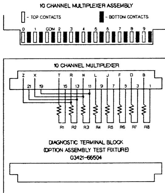
The resistance of each channel (0-9) on the card is checked sequentially, using the 2-wire ohms function. Channels 0 and 1 are first checked to see if they are actuators. If they are actuators, the actuator channel
