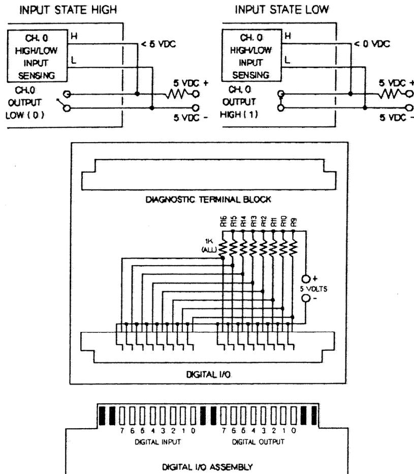
When the test begins, the program opens all channels in the instrument. With all of the channel outputs on the card open (set to the low state), the 5 Vdc supply, sensed through the DTB pull-up resistor for each channel, should set a high state on each channel input.
