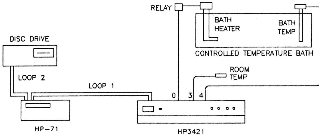
Figure 8-1. Temperature Logging System With Actuator Control
