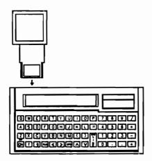
The adapter plugs into the HP-IL port at the back of the HP-71. First slide the cover off the port, then insert the adapter. Be sure the slot in the end of the interface is towards the bottom of the computer. Push in the adapter until it snaps into place.
