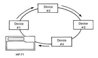
If any device isn't turned on, it will probably disrupt the operation of the HP-IL system because it can't pass messages around the loop.
