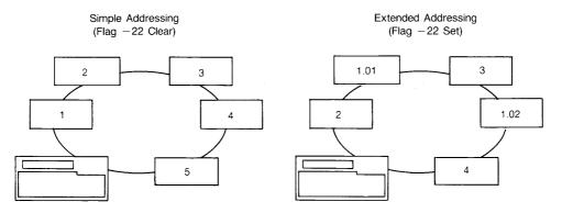
If you use ASSIGN IO to establish assign codes for HP-IL devices, the HP-71 automatically uses simple addressing—the setting of flag -22 is ignored. Simple addressing is used until all assign codes are cancelled by ASSIGN IO \*—then flag -22 determines the addressing scheme.
