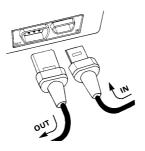
If any HP-IL device is turned off (and it can't be turned on by the HP-71), it will prevent HP-IL operation.
