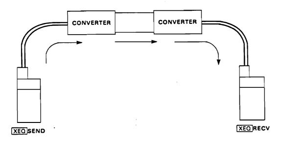
The following program is stored in each calculator. Execute RECV on the calculator that is to receive ALPHA data, and execute SEND on the calculator that is to send ALPHA data. Then enter a message at the sender followed by R/S.
