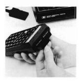
3. Insert the printer interface module into the empty port as shown. Push it into the calculator until it snaps firmly into place.
