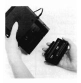
Insert the new battery pack so that its contacts face the printer and line up with the connector springs.
