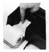
Press the paper advance key and hold it down until the paper passes the top of the plastic tear bar.
