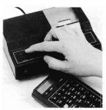
2. Remove the port cap that is in the highest numbered unused port. If you must remove a memory module, always remove one from the highest numbered port. (If you remove a memory module, make sure the HP-41C has enough memory allocated to data storage registers—executing SIZE 064 will ensure this.)
