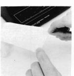
Temporarily place the paper roll in the paper roll cover. With your finger, push the leading edge of paper into the slot near the bottom of the paper well. Continue pushing until the paper can be pushed no further into the print mechanism.
