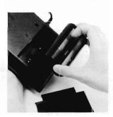
5. Insert the end of the battery door that is opposite the latches behind the retaining groove, and close the door.
