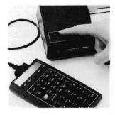
Pull the printer interface module straight back until it is free from the port. Do not pull on the cord.
