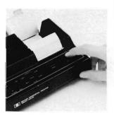
5. Drop the roll of paper into the paper well, close the cover, and press PRINT two or three times. (If you ran out of paper during the execution of a program, press R/S.) If the paper is feeding properly but no printing appears when you print, the paper may be inserted backwards. The paper is chemically treated and will print on only one side.
