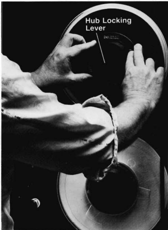
Figure 3-5. Mounting the Supply Reel
