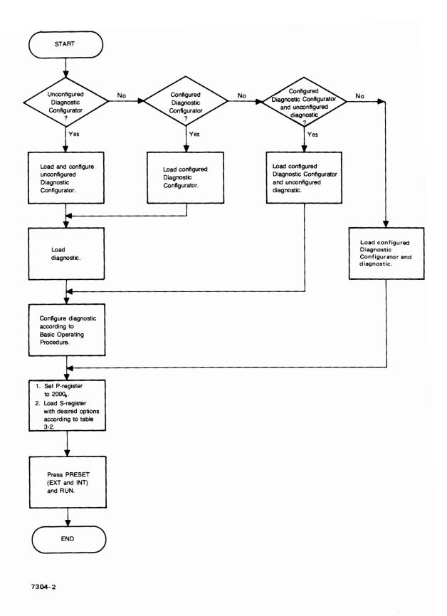
Figure 3-1. Load/Start Procedure Flowchart
