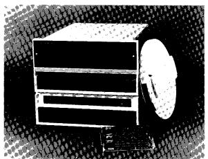
HP's latest high performance disc storage subsystem offers both increased thruput and capacity. The 12962A consists of a 15 megabyte disc drive, Storage Control Unit, and interface card for a 2100/21MX Series CPU. The drive and Storage Control Unit (SCU) have built-in power supplies. Only one I/O slot is required to interface to a 2100/21MX Series CPU.
